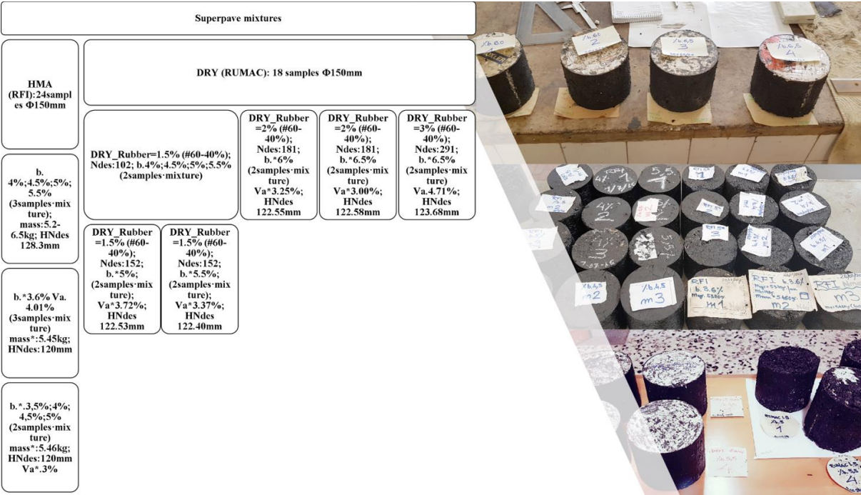
Fig. 11. (a) Materials and mixtures specifications on this research; (b) HMA_DRY Specimens developed
