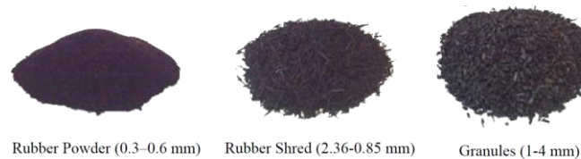
Fig. 15 Difference sizes of crumb rubber used
