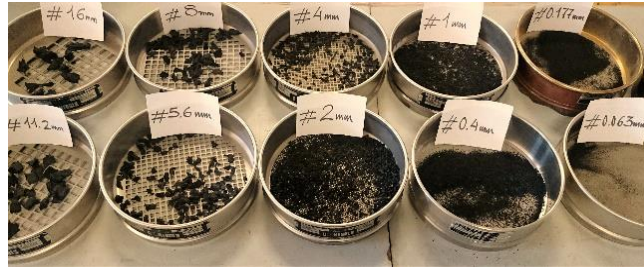
Fig. 6 Sieve analysis of the rubber from discarded truck-tires
