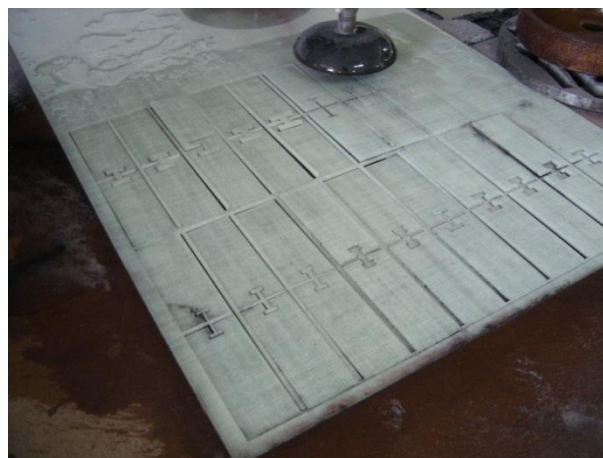
Fig. 3: Specimen cutting with water jet.
