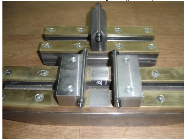
Fig. 7: Manufactured three-point bending apparatus
