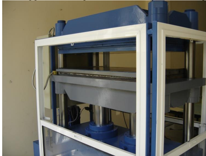
Fig. 1: Composite material-manufacturing press.
