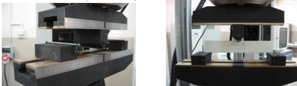
Fig. 10: Three-point bending experiment.
