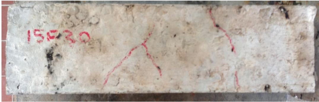
Figure 12: specimen after heating (300°C) in oven for two hours
